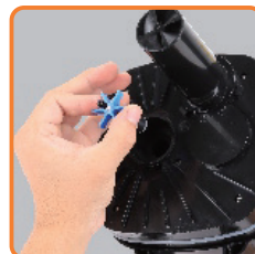
FIG2: Take out the impeller for cleaning
